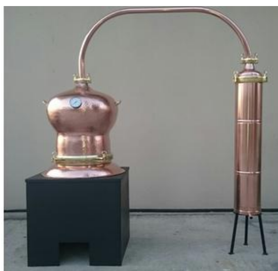
Picture 2: Traditional alembic: (1) kettle, (2) cover, (3) cooler (serpentine), (4) distillation receptacle, (5) heater.
